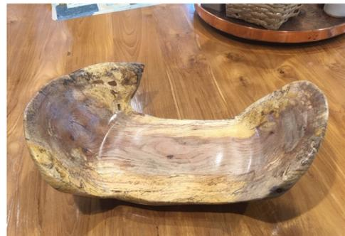
**FINISHED BOWL PIECE, COATED WITH SANDING SEALER, LATEX OVERLAY, AND WAXING.**
