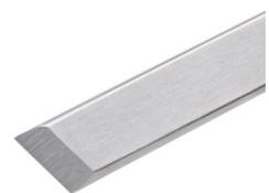
degree point. Don't worry about the rake, but 15 degrees is good enough. The cutting edge is not flat, but rather curved outward, or convex. How does this work? The raised bevel (bump) rides on the stock while the edge contact is controlled by you twisting your wrist. Not raising your arm, shifting your weight or picking up one foot; all you do is twist your wrist.
