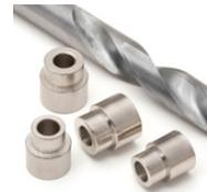
The size of the material where the nib, band, cap, clip, etc makes contact is governed by the bushing. Kits use different bushings for different mandrels. Stick with a style until you can run with the big dogs, then just go for it.
